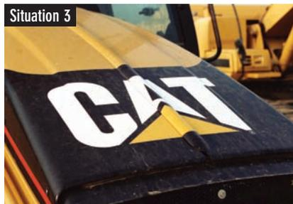
rior use, polyester is a plastic material typically used for membrane switches, overlays and nameplates. It's heat-resistant and stable and won't stretch or shrink, but it doesn't form over surface irregularities like vinyl. Polyester can be coated with permanent pressure-sensitive acrylic adhesive.
